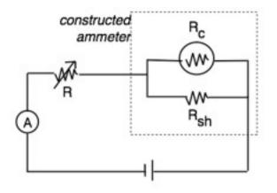
To check your constructed ammeter, you are going to measure the same current using two ammeters, the constructed ammeter and the commercial ammeter. Adjust the rheostat so that you measure some current (up to your choice) lower than the maximum current that can ben measured with the constructed ammeter, that is, lower than 6.0 A. Record your readings from the constructed and commercial ammeters in Table 2 given below in the "Data and Results" section.
