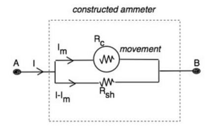
In the figure, I is the current that is to be measured,  $I_m$  is the current passing through the movement, so the current passing through  $R_{sh}$  is I-I<sub>m</sub>. Since the movement and the shunt resistance are connected in parallel, the potential difference on each of them is the same and is equal to the potential difference between points A and B. That gives:
