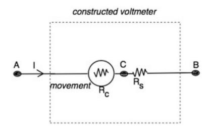
Here, the same current I passes through both the movement and the additional resistance. However, if  $R_s$  is much larger than  $R_c$ , than the potential difference between points A and C will be much larger than the potential difference between C and B. Since:
